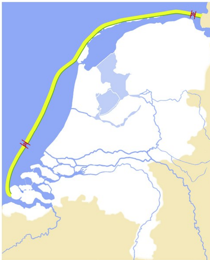
Figure 32. The forward approach: building a dike some 30 kilometres off the coast to protect against floods from the sea. [Source: Vellinga (2008) 40 ]
